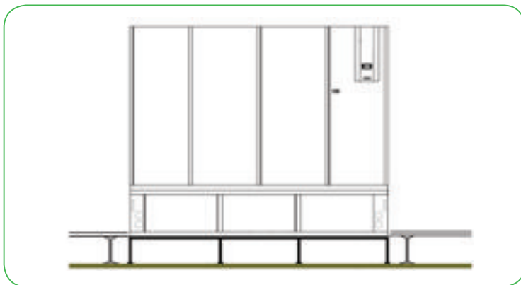
Unit with fan plenum installed above the raised floor
